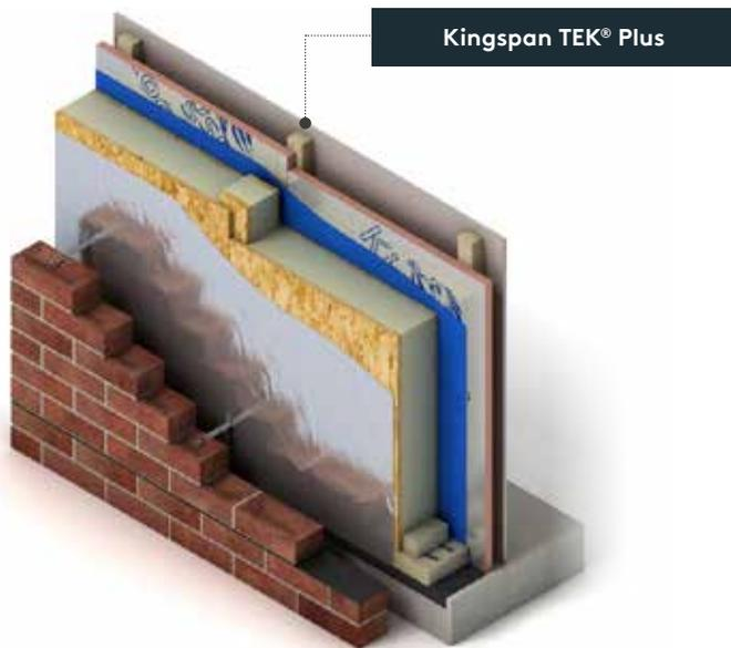
Kingspan TEK® is our structural insulated panels (SIPs) building system. It's manufactured in a quality-controlled factory to a design that matches your architectural plans. By choosing the Kingspan TEK® building system, you can achieve thermal performance levels as demanding as those required by the Passivhaus standard.
